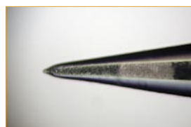
Figure 2 PicoFrit® column packed with ProteoPep™ II C18; 5 \mu\text{m} bead, 10-cm bed
