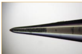
Figure 4 PicoFrit® column packed with ACQUITY™ C18; 1.7 \mu\text{m} bead, 10-cm bed
