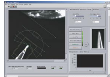
Figure 4 - The ROI are defined by the user in the automatic controls tab
