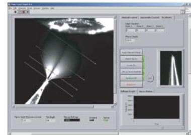
Figure 5 - Spray analysis of the multi-jet mode. The number of edges in each ROI and with the plume angle are shown in the readout tab
