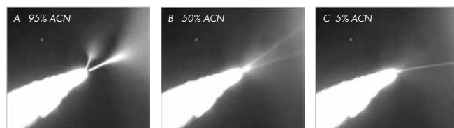
Figure 4 ESI plume photos at 95%, 50%, and 5% ACN, respectively. The flow rate was 500 nL/min. 15 µm PicoFrit emitter with an applied voltage of 1.8 kV.
