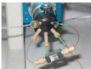
Figure 9 Union is inserted into the autosampler injection valve
