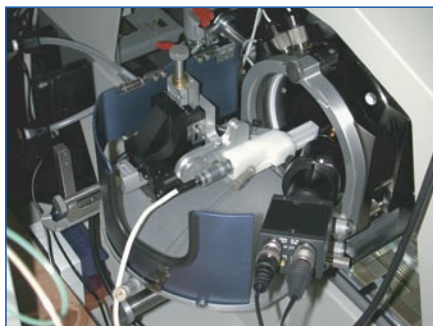
Nanospray source configured to use conventional capillary columns and coated fused-silica tips. HV is applied directly to the tip.
