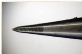
Figure 3 PicoFrit® column packed with HALO™ C18; 2.7 \mu\text{m} bead, 10-cm bed
