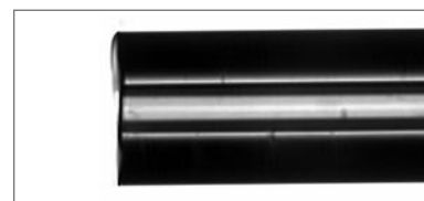
FIGURE 11 Typical cleave. Polyimide coating was removed after cleaving for clarity of image.
