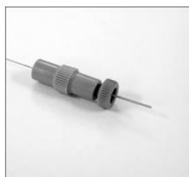
FIGURE 7 Column tip pulled back into sleeve
