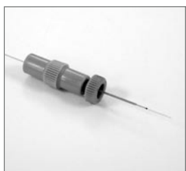
FIGURE 6 Column pulled through sleeve
