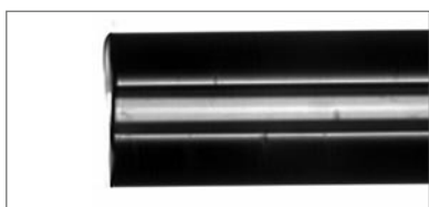
FIGURE 12 Typical cleave. Polyimide coating was removed after cleaving for clarity of image.
