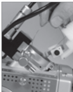
FIGURE 10: Insert the probe into the port after positioning the column inside
