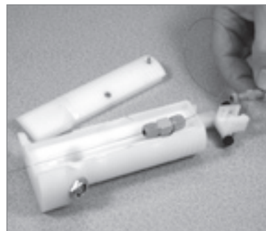
FIGURE 6: MicroTee in Position A for short columns
