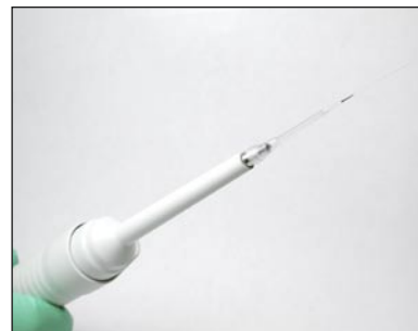
Figure 2 Trap'nTip™ fitted onto 10 µL pipette
