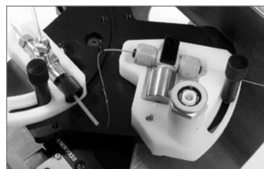
Figure 5 UTM in rear stage position loaded with the MicroTee
